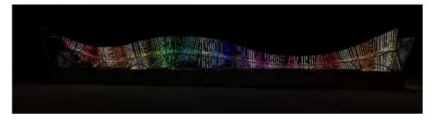
If possible it can be only translucent strip incorporate with LED lighting system programing for special lighting. Some events might use this lighting float and run on glass roof to create activities atmosphere at the parking area (multi purposed area). So the color of strips will be flexible not only one color at one position, but it can also be changed in 195 sticks.
